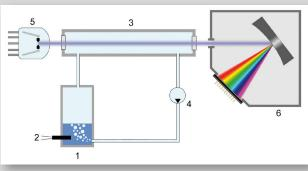
1: stripping pot, 2: temperature probe, 3: gas flow cell, 4: gas pump, 5: xenon flash lamp, 6: spectrograph
