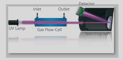
The measuring principle is based on the UV light absorption according to the Beer-Lambert Law:
